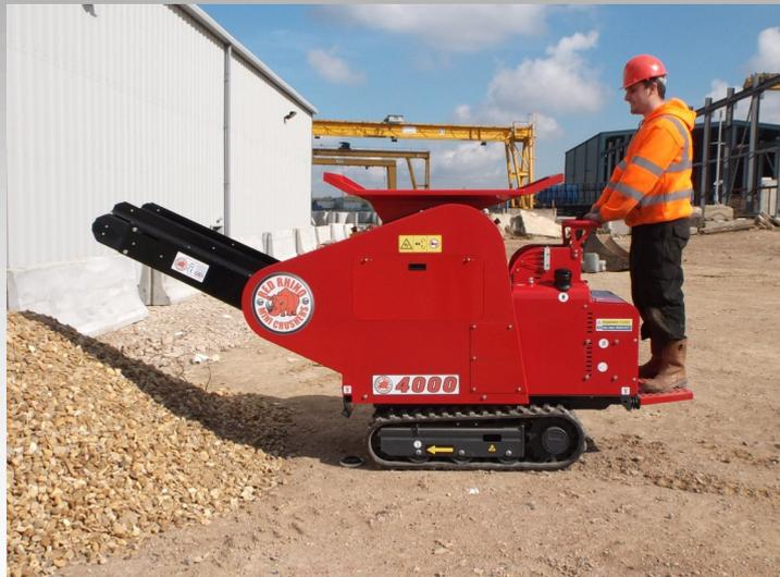
Electric start with clear and simple hydraulic controls.
